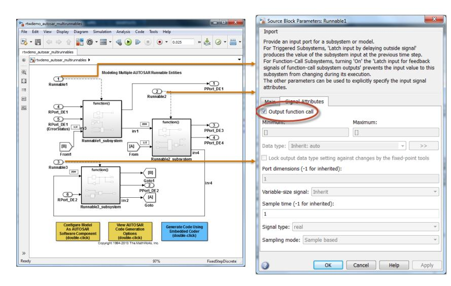
For the multi-runnable modeling pattern, each input port that represents a runnable trigger event will need to have the check box for Output function call checked as part of the inport properties.
