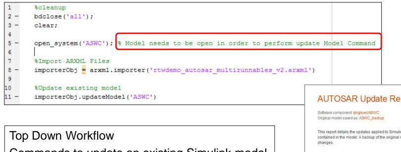
Commands to update an existing Simulink model that already has an AUTOSAR configuration.
