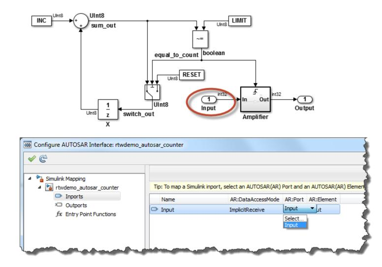
Here is an example of mapping a Simulink Inport to a AUTOSAR Port Data Element. In this case, you can see the Simulink Inport called Input is mapped to the AR:Port of Input. The actual selection of the AR:Element is a bit hidden in this view. Notice that the AR:DataAccessMode is also available for the user to select from this dialog.
